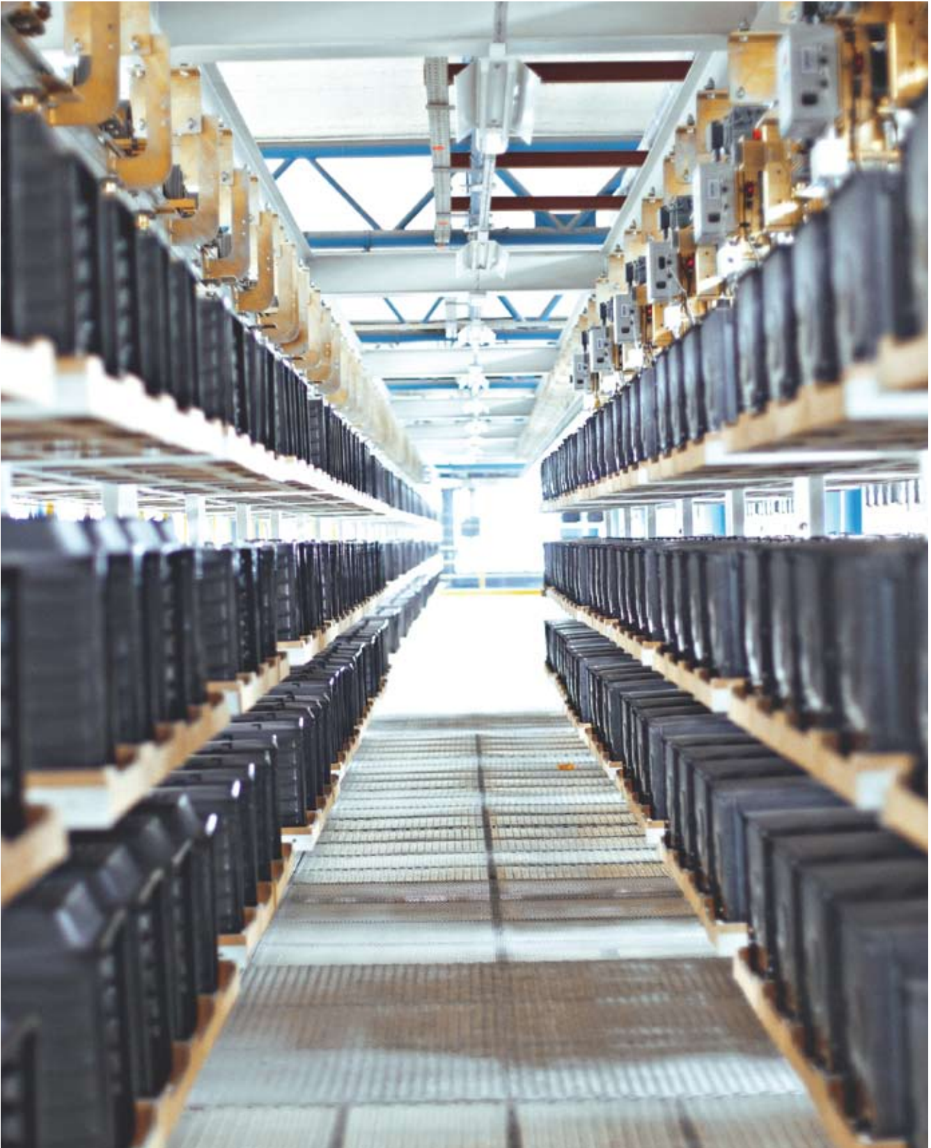
Buffer storage of enamel coated ovens waiting to proceed to the assembly/fitting lines at the Cooking Appliance Program. The buffer is a part of the transport system used to convey enamel-coated ovens from the enamel coating plant to the assembly lines.
